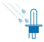
Only a burning bulb made of quartz glass (filament 2650°c, glass 800°c) can resist thermal shocks: such as, if a drop of cold water touches the hot bulb, when you drive through water with a broken headlight unit.
